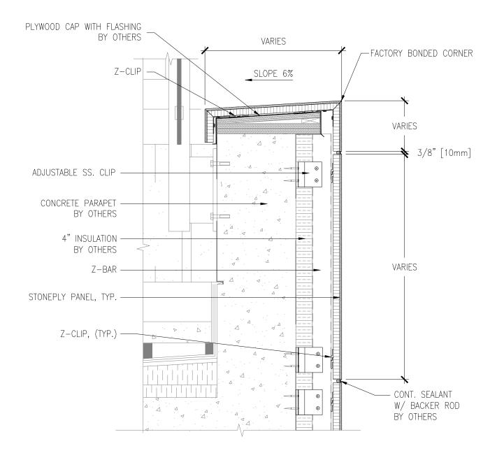
PARAPET DETAIL WITH STONEPLY CAP
