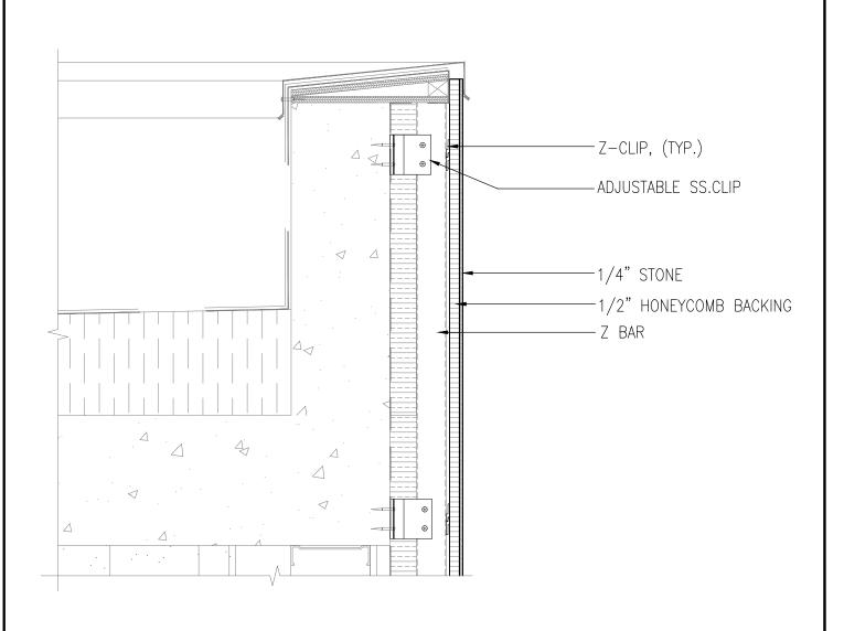
PARAPET DETAIL WITH STONEPLY AND METAL CAP SCALE: 1 1/2"= 1'-0"
